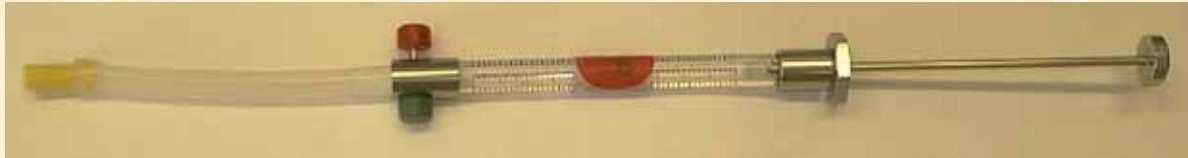
Syringe/tubing dissolved gas sampler.
