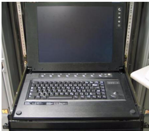
Figure 4. The KVM and monitor, for local user access.
