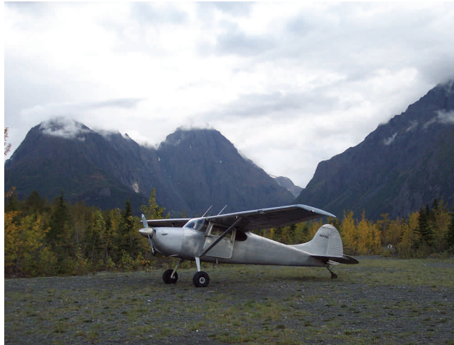
Cessna 170B modified with Lycoming O-360 engine, constant speed propeller, STOL Wing, heavy duty landing gear, and avionics upgrades
