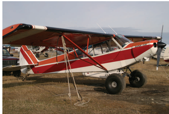
Piper PA-18 modified with belly pod and large tires
