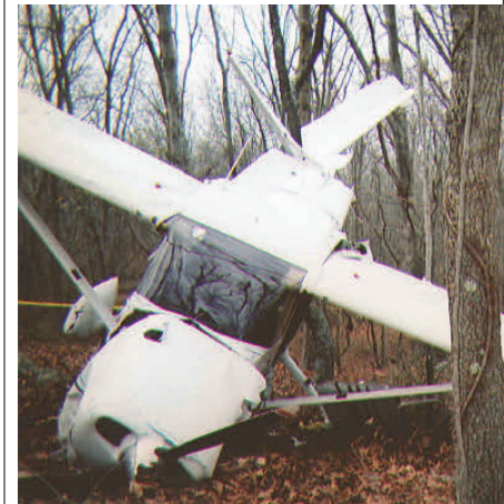
Airbags deployed and both occupants received only minor injuries. Photo courtesy of AmSafe.
