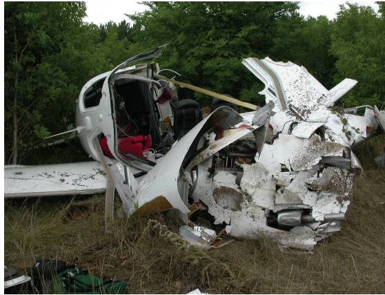
Aircraft stalled and cartwheeled. The aircraft was destroyed, but the airbags deployed and the occupants evacuated without life-threatening injuries. Photo courtesy of AmSafe.
