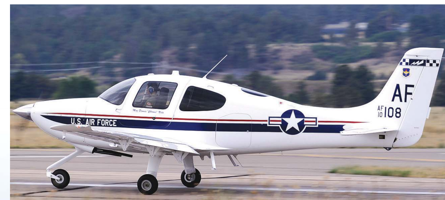
Left: The Cirrus Aircraft T-53A is a small, single engine aircraft at the Academy that replaced the fleet of Diamond DA-40 T-52s in the spring of 2012. It is slightly larger than the T-52 and has a slightly higher horsepower engine. It provides exposure to powered flight and gives cadets the opportunity to solo.
