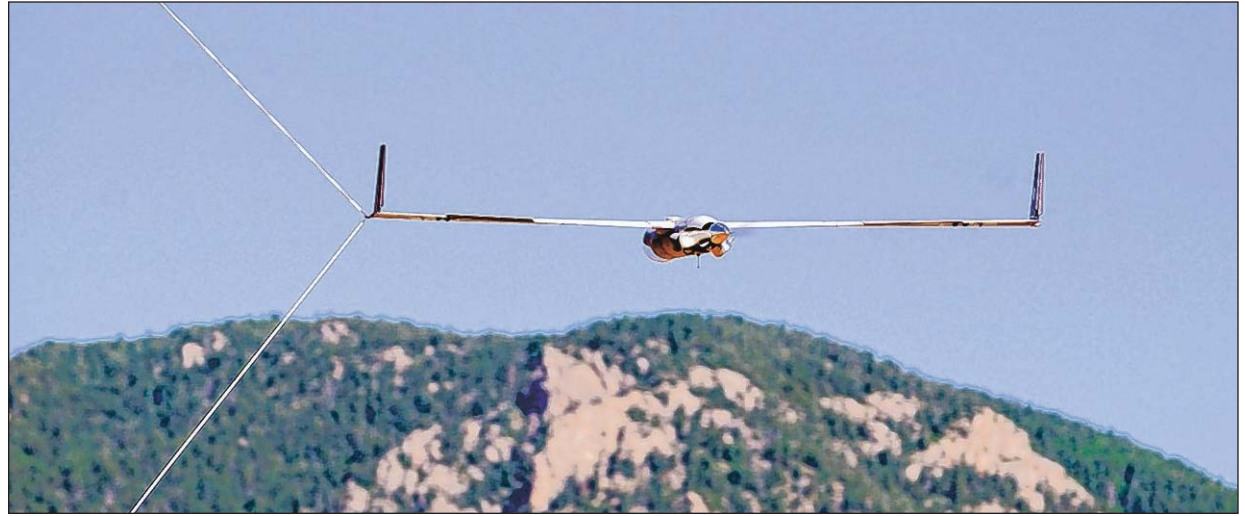
A ScanEagle remotely piloted aircraft snags a capture cable during an Air Force Academy Airmanship 200 lesson at Fort Carson July 6.
