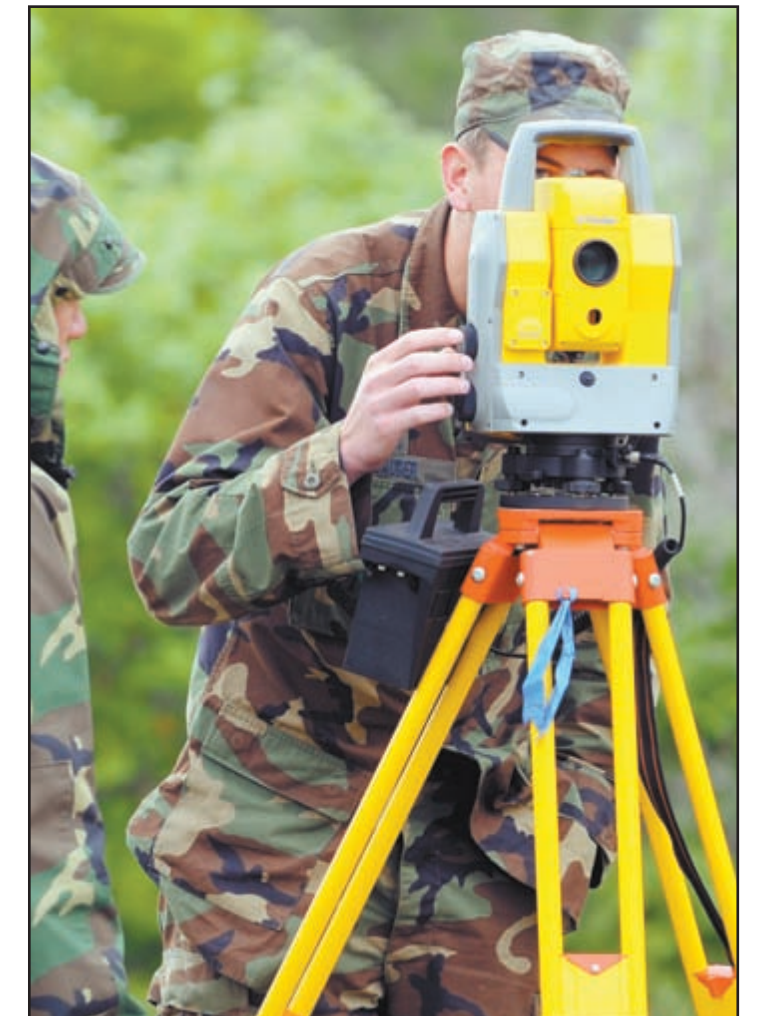
Cadets used the total station in one of the surveying activities.
