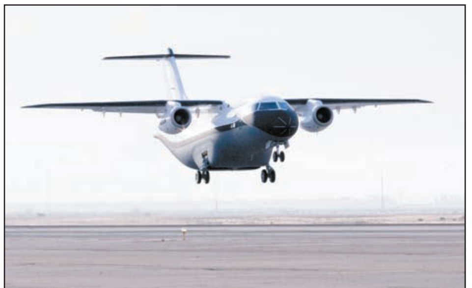
The Advanced Composite Cargo Aircraft made its first test flight Tuesday from Air Force Plant 42 in Palmdale, Calif. The ACCA is proof of concept technology demonstrator for advanced composite manufacturing processes in a full-scale, certified aircraft.
