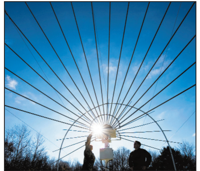
Photo by Lance Cheung Master Sgt. Yolanda Hernandez, left, and Staff Sgt. Stephen S. Ensminger, electronic systems maintainers, stand under the sweeping dipoles on a Solar Radio Spectrograph. The SRS measures radio wavelengths between 25-75 MHz.
