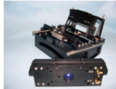
Brassboard camera with dual photoelastic modulator assembly in the foreground. (This multi-angle UV/V/NIR polarimetric spectrometer has been developed through prior ESTO IIP.)
