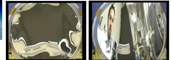
An optical quality PVDF film deforms from a flat shape to a concave shape with the application of the voltage
