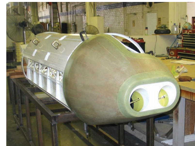
Assembly of the first SAR pod, to be flown on the NASA Gulfstream III aircraft, viewed from the aft end of the pod. Note the two aft cooling ducts; these are critical to maintain the antenna and equipment at an appropriate temperature.
