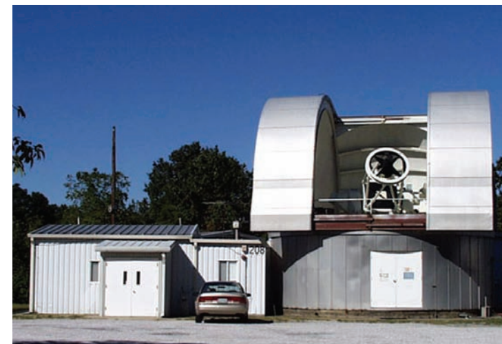
Goddard technologists used this 48-inch telescope tracking facility at the Goddard Geophysical and Astronomical Observatory to transmit the 20 mJ laser return signal to the MESSENGER spacecraft
