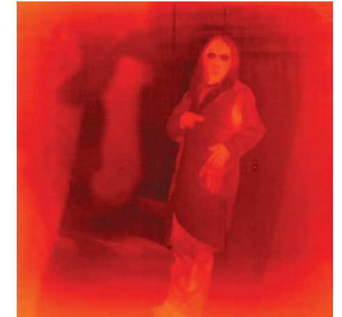
A false color image of a NASA engineer in the far infrared taken with the one megapixel QWIP camera. Warmer temperatures are orange, cooler temperatures are dark red. Notice the thermal handprint on her lab coat as she removes her hand from her pocket.
