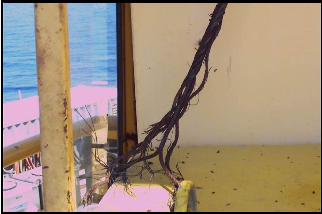
Figure 24 – End section of failed boom hoist wire rope
