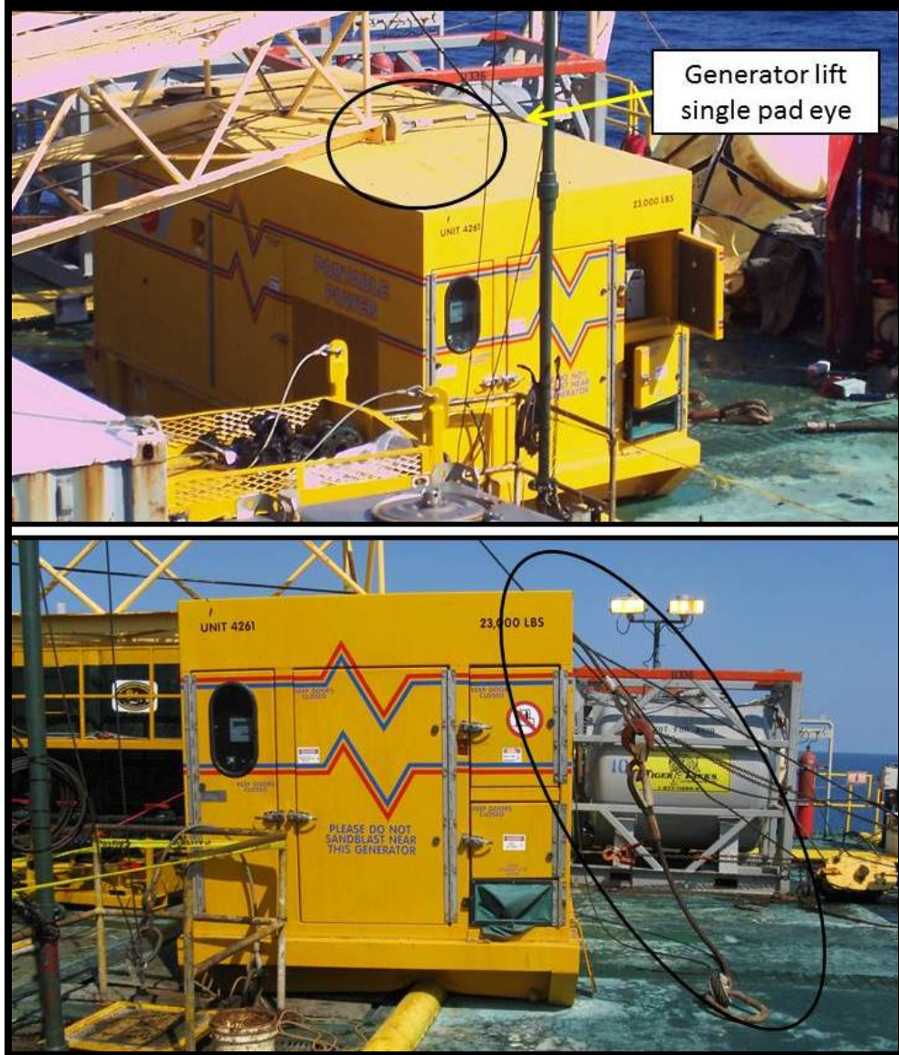
Figure 10 - Generator lift point and rigging, post-accident
