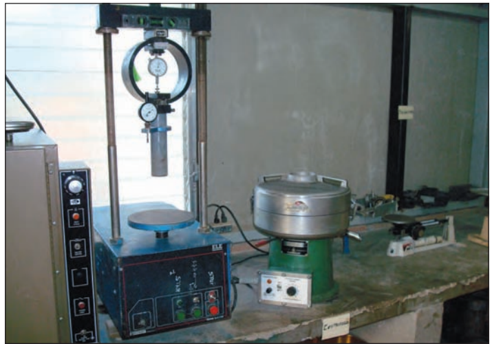
Soil strength testing equipment
