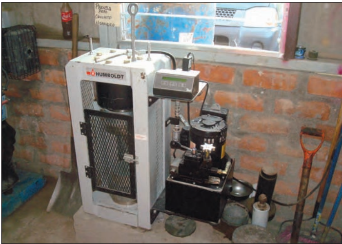
Concrete strength testing equipment
