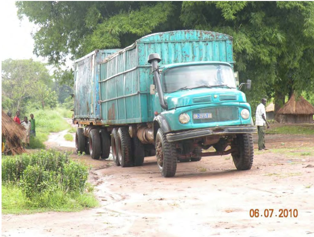
This Congolese-registered truck on Ngangura-Nabiapai Road demonstrates the need for a mechanism for axle load controls on the improved roads (Note: It took the truck 6 hrs to move the 13 km from the DRC border to here)
