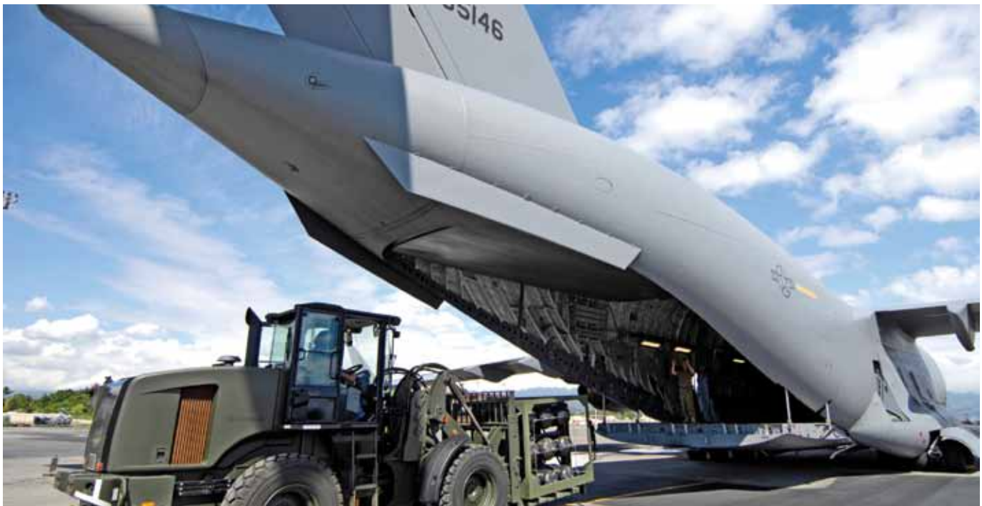
The HydraFLX System is brought up to the back end of a C-17 Globemaster III to demonstrate its mobile capability at Hickam Air Force Base, Hawaii. The Air Force is testing the HydraFLX System as an alternate energy source. It will generate ultra-pure H2 (hydrogen) from water in a flexible pressure management process for fueling buses, tow-tractors, vans, sedans, and ground support equipment. The system can also be deployed anywhere and operate in hostile theaters without infrastructure or pipelines.
