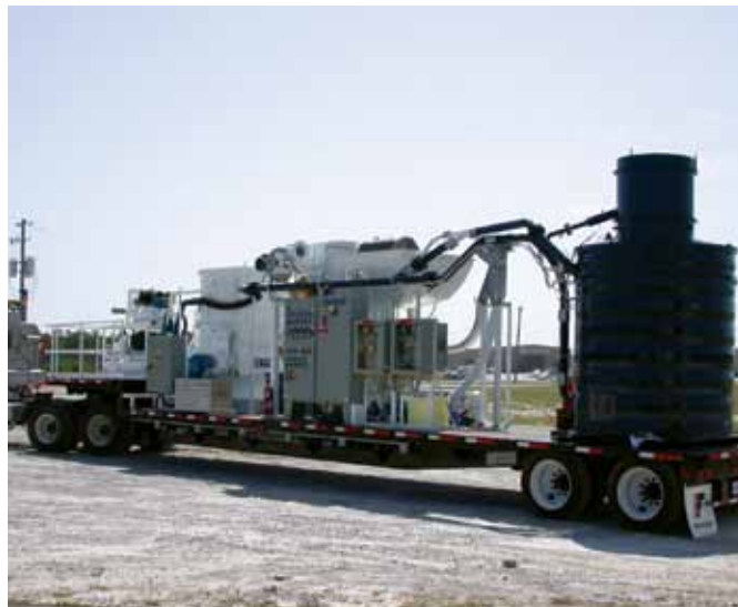
Researchers at Tyndall Air Force Base, Fla., have designed a transportable waste-to-energy system, shown here, that will use waste material to produce electricity at forward-deployed locations.
