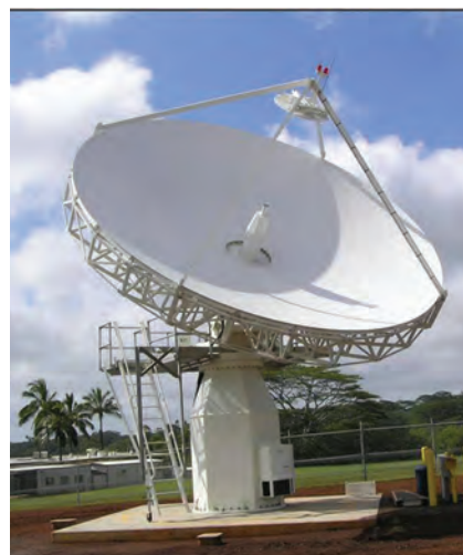
AN/GSC-70 Ka-Band Satellite Transmit and Receive System (Ka-Stars) Terminal, Wahiawa, Hawaii.
