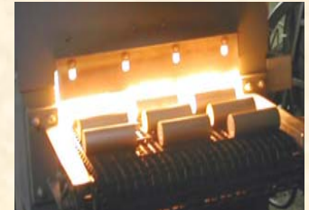
Preheating of Aluminum Billets
