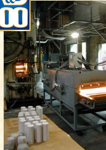
Full-scale Production Based Infrared Furnace operating at Queen City Forging Company
