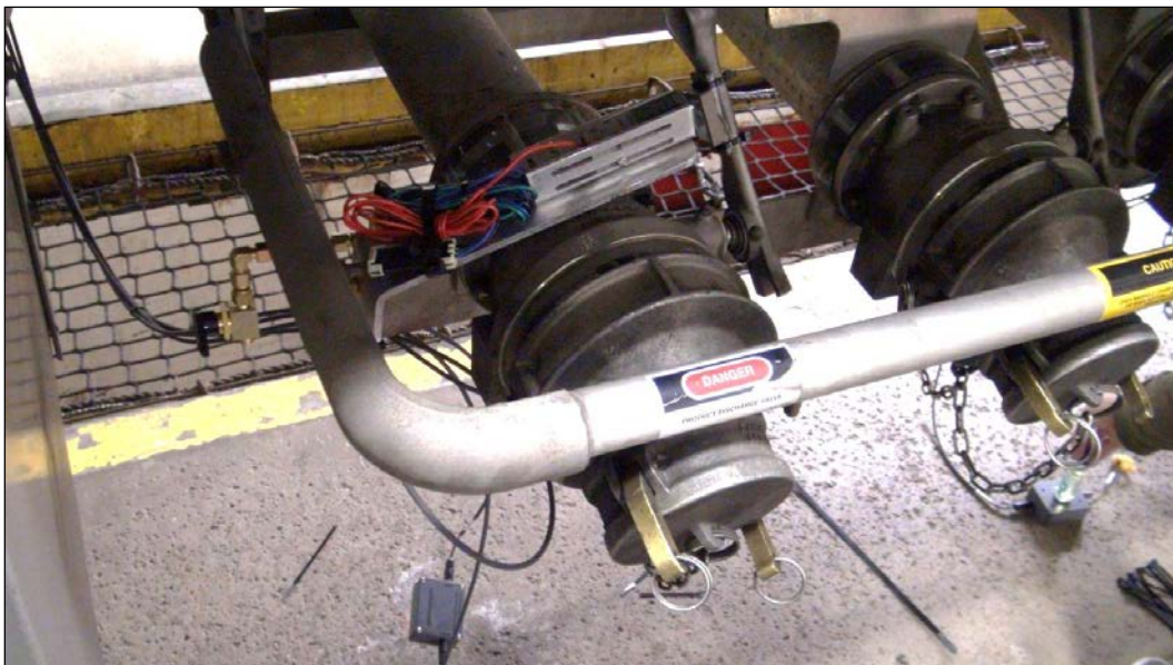
Fig. 90. Instrumented valve on tanker.
