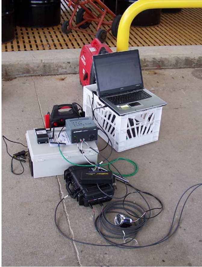
Fig. 81. DAS and T2TCU testing with fuel loop.
