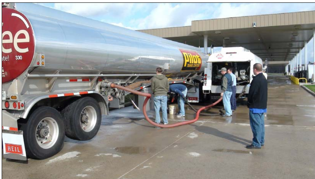
Fig. 92. Test vehicle connected to TRC tanker for fuel transfer.
