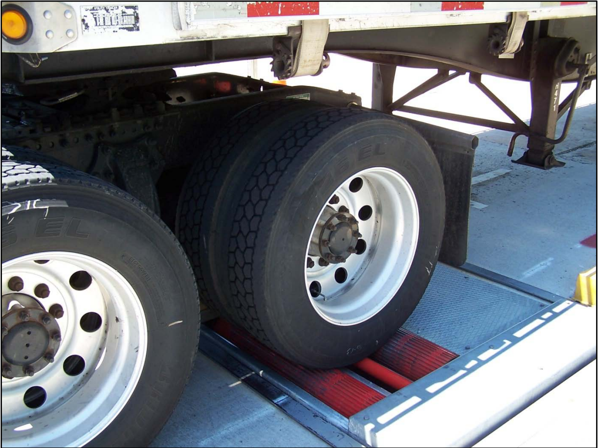
Figure 4. Performance based brake tester, located at Greene County Inspection Station.
