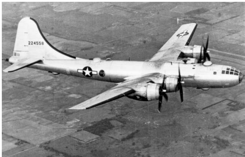
The B-29 Superfortress. The aircraft, available for deployment in 1944, was the largest and most advanced bomber of World War II. The “Superfort” had a 141-foot wing span and a combat radius of 3,259 miles. It provided the very long range that the Army Air Corps realized in the late 1930s would be required over the vast Pacific.
