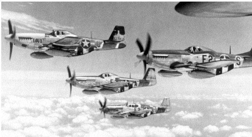
P-51 Mustangs over Europe. Drop tanks made all the difference, providing greater range to these and other types of fighter escorts as they protected long-range bombers against enemy aerial attacks.
