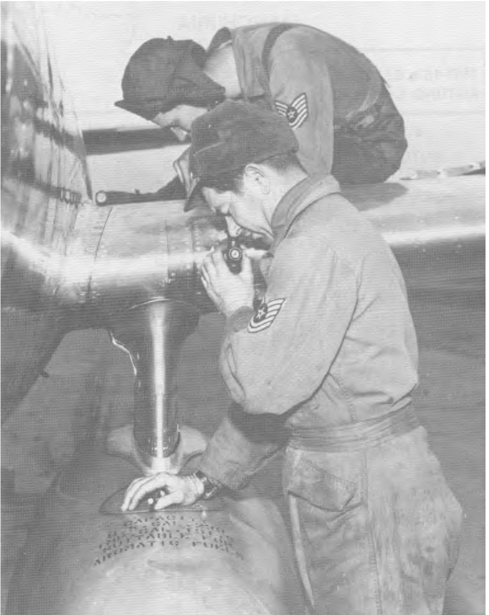
Crewmen boresight the wing gun of an F-84.
