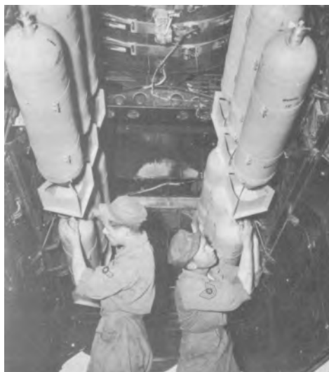
Armament technicians insert the nose fuses into photo-flash bombs used on RB-26 night reconnaissance missions.
