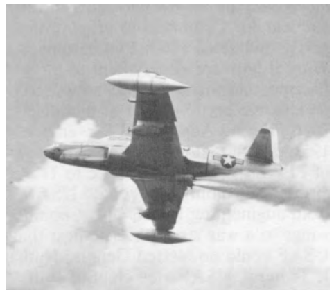
A JATO-equipped F-80 takes off with a 500-pound demolition bomb nestled beneath each wing.
