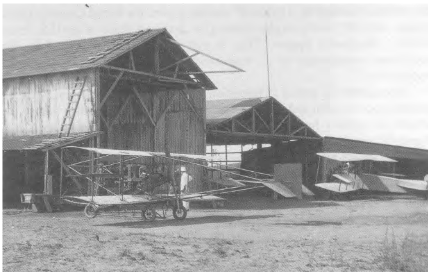
The hangars at North Island with two Curtisses parked outside. The pusher Model E is at the left, and the tractor Model G is to the right.
