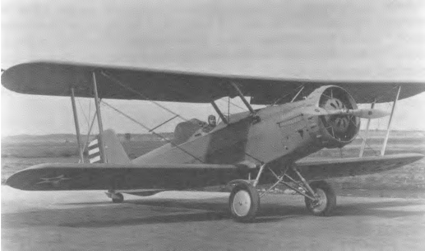
An early model BT-2 equipped with a blind flying hood appears above.
