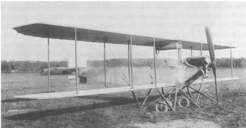
The Burgess H tractor, a weight-carrying Scout, with Wright lever controls
