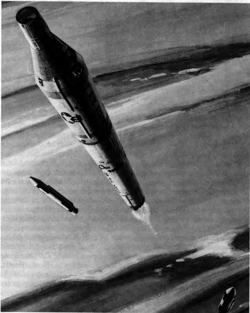
Artist's concept of a MOL-Titan IIIC launch. The solid-propellant boosters have separated and are falling away. The two-man crew in the Gemini spacecraft atop the stack, would transfer to the orbiting laboratory module (beneath it) for a 30-day mission.
