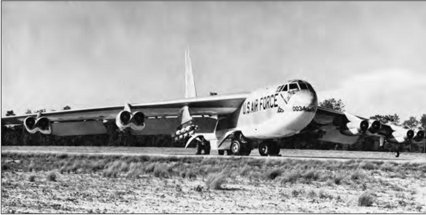
A SACB-52 carries a load of conventional (nonnuclear) bombs hanging beneath each wing. All B-52 bombers were capable of carrying nuclear or conventional bombs to any target in the world.
