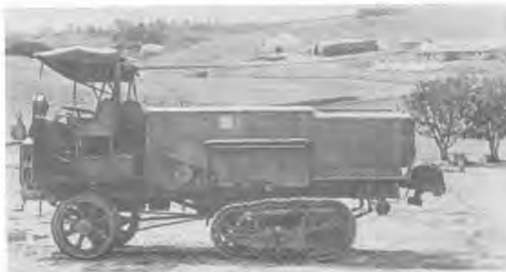
A balloon windlass mounted on a truck with a caterpillar adapter.
