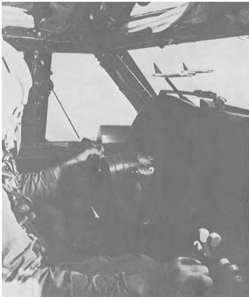
View from the cockpit of the third aircraft in a three-ship right echelon formation. This was the basic formation used for in-flight refueling as the bombers approached their tankers.
