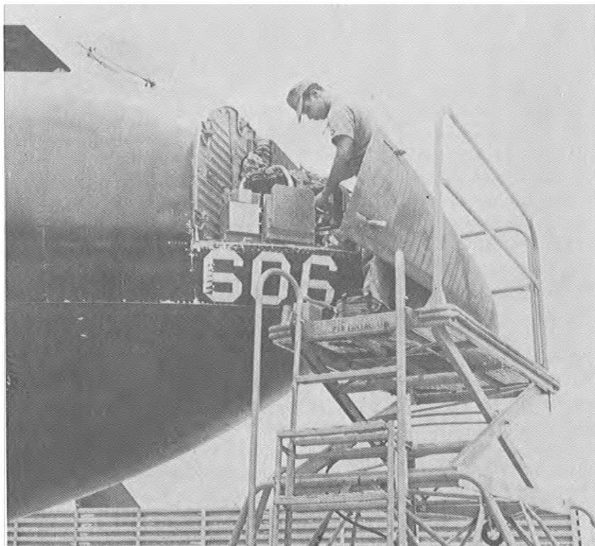
A specialist concentrates on repair of electronic components in the nose of a B-52D.
