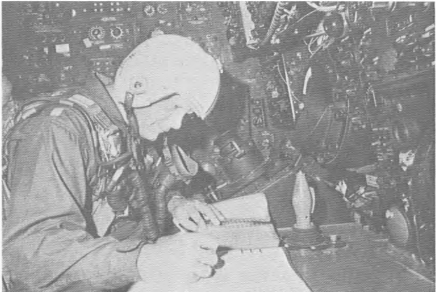
Major Robert A. Hewston, radar navigator veteran of three LINEBACKER II missions, cross-checks mission data at his downstairs position, nicknamed the “Black Hole of Calcutta.” His cramped work area and maze of equipment are typical of B-52 crew positions.
