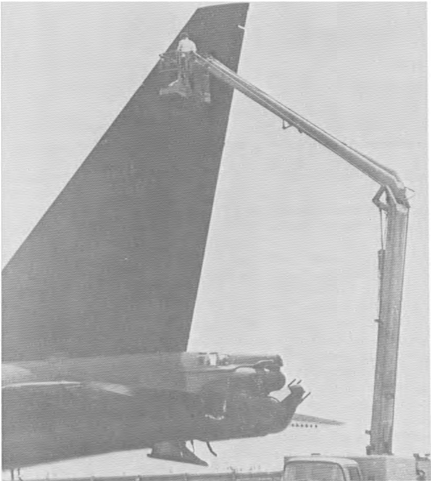
The tall vertical stabilizer of a B-52D dwarfs a maintenance technician in a "cherry picker."
