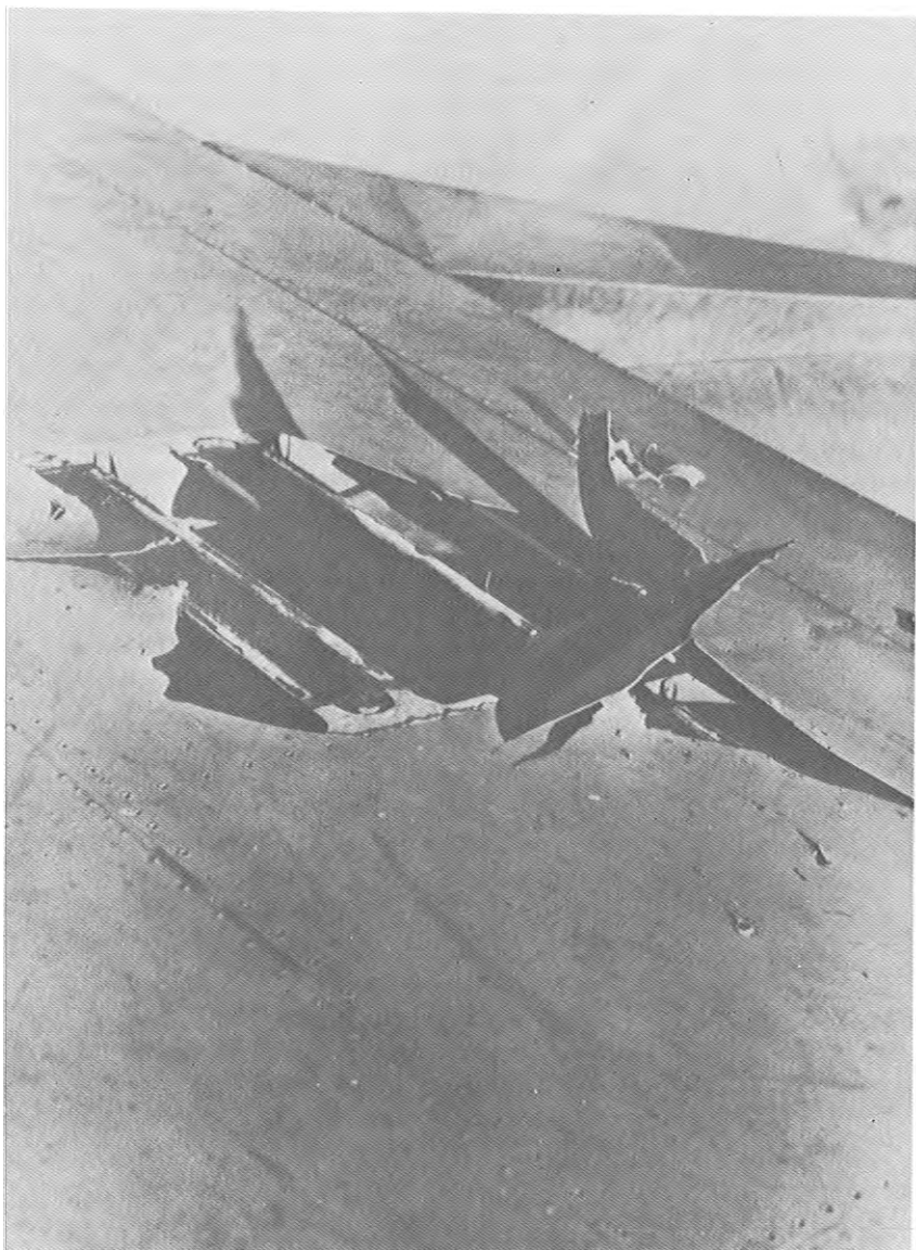
The hydraulic ram force of SAM fragments, with an estimated penetrating capability at 75 feet at least equal to a .50 caliber all-purpose round at muzzle velocity, is evident on this upper wing surface.
