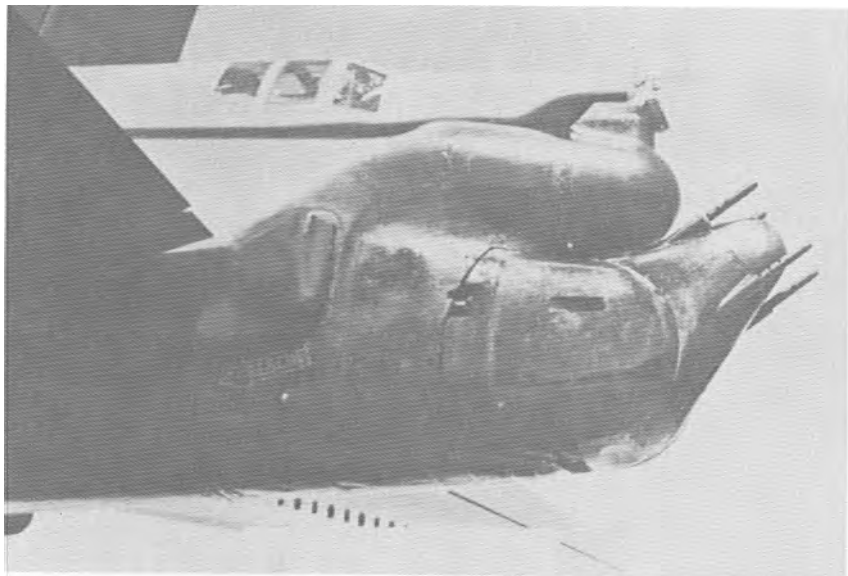
Close-up view of the "D" tail gun system. Guns were pointed up during maintenance. The gunner's canopy resembles fuselage-mounted pilots' canopies of older style aircraft. For bailout, the turret is jettisoned at the seam just aft of the canopy.
