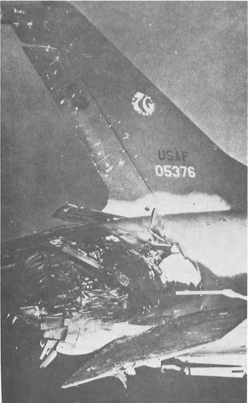
An F-105 after being hit by an air-to-air missile. Booster is visible imbedded in aircraft tail section.
