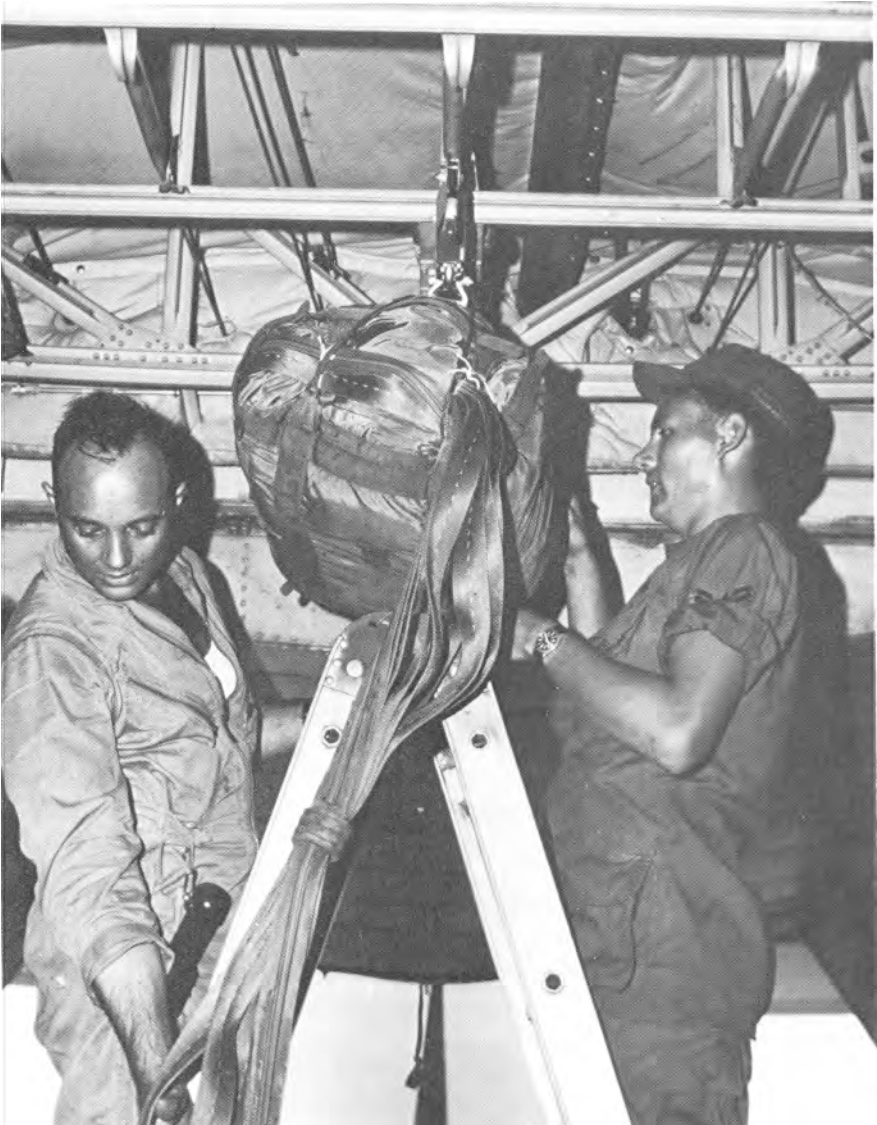
Two airmen aboard a C-130 rig a pallet of cargo and parachute extraction equipment for a low altitude drop, June 1967.
