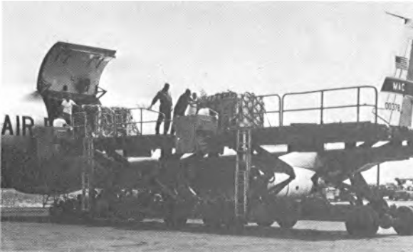
The adjustable 25K-loader has roller tracks, cutting the unloading time for this C-135 from hours to minutes, Tan Son Nhut, 1966.
