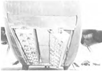
Arc lamps mounted under a C-123 provide a constant light source with a two-mile diameter, when the aircraft flies at 12,000 feet altitude.
