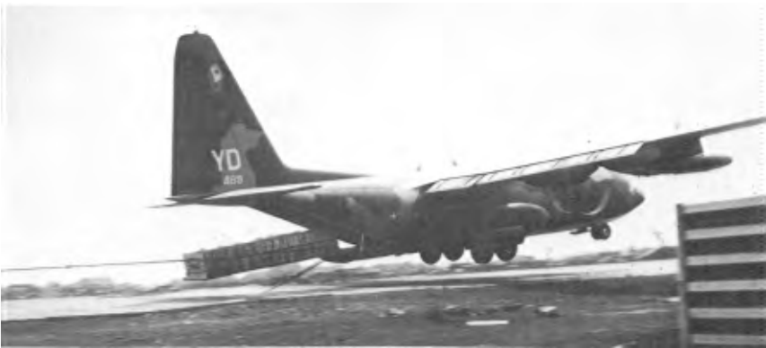
The trailing hook of the C-130 cargo load catches on the arresting cable stretched across the Khe Sanh runway. The technique, called the Ground Proximity Extraction System, was used successfully at Khe Sanh to decrease the aircrafts' exposure to enemy fire and ensure accurate cargo deliveries.
