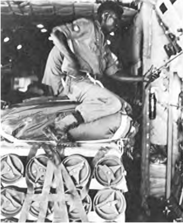
An Army rigger aboard a USAF C-130 attaches a static line to a hook-up cable, getting ready for a cargo drop to the Marines under siege, March 6, 1968.
