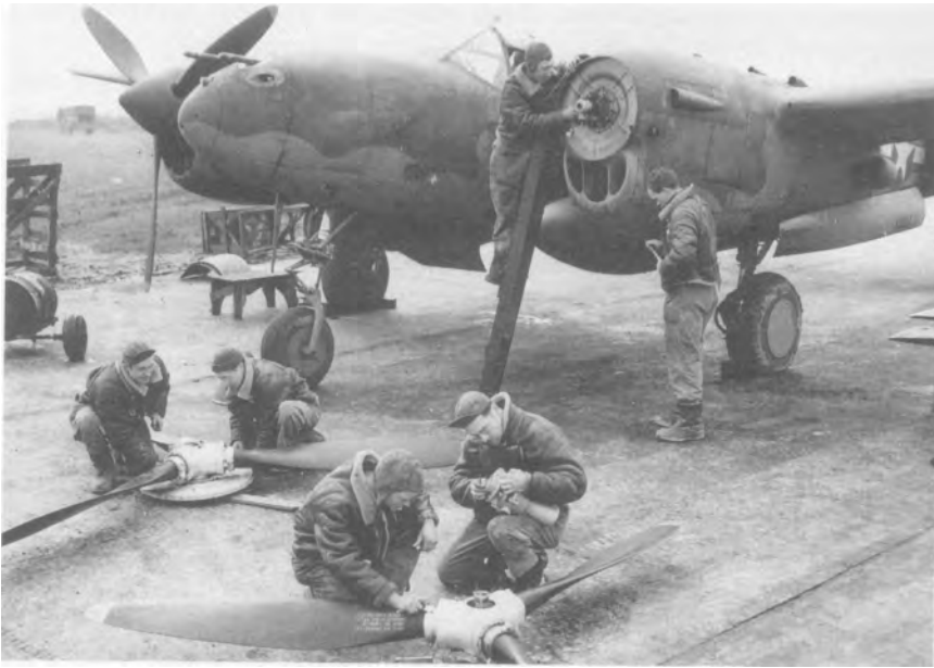
Eighth Air Force ground crews servicing a P-38. They worked unprotected from the elements, often at night.
