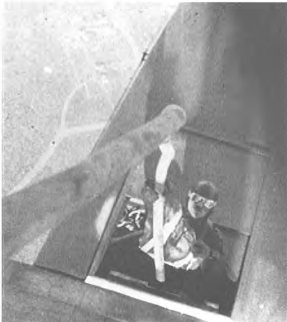
The Question Mark Flight, January 1929. Scenes from the aerial experiment. Clockwise from above: The interior of the Question Mark reveals the positions of an auxiliary gas tank on the floor, refueling apparatus on the roof, and berths. A chase aircraft with its chalked message ( opposite, above ) shows one means of communication before the introduction of reliable airborne radios. The gravity-fed transfer of gasoline proceeds between aircraft ( opposite, below ). Spatz ( below ) wrestles with the refueling hose as it reaches the Question Mark .
