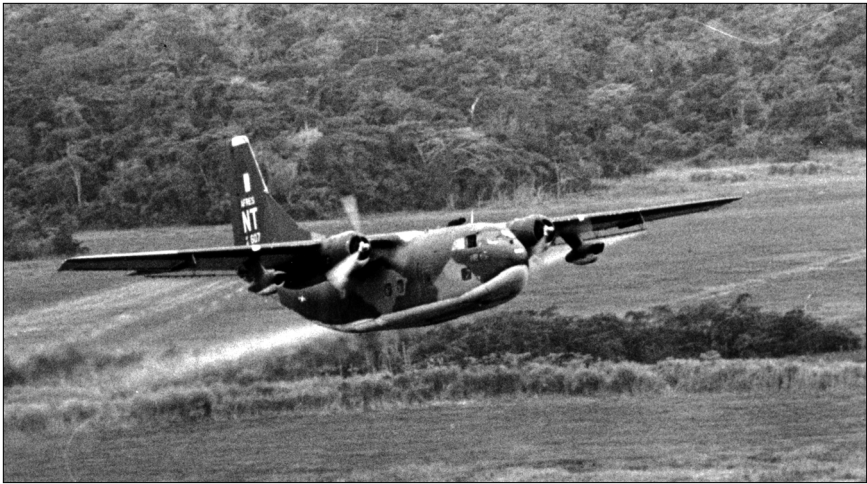
A C-123K sprays insecticide over salt marshes in the Canal Zone to control mosquitoes spreading deadly disease in the area. (NARA photo.)
