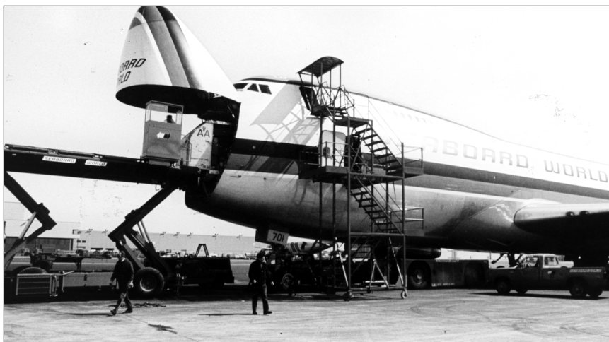
An extending loader is used to load medical and relief supplies onto a commercial contract 747 for airlift to Zaire. (NARA photo.)
