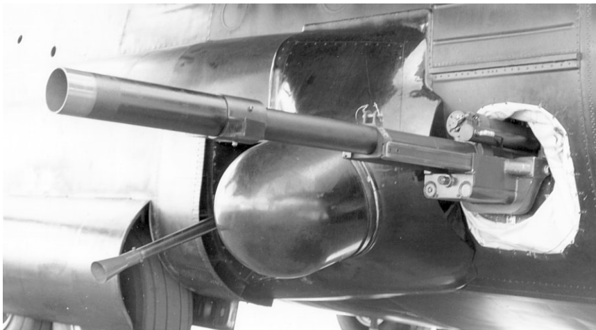
The left side of an AC-130 with a 105-mm howitzer and a 40-mm gun. In between is the tracking radar that directs the two guns.
