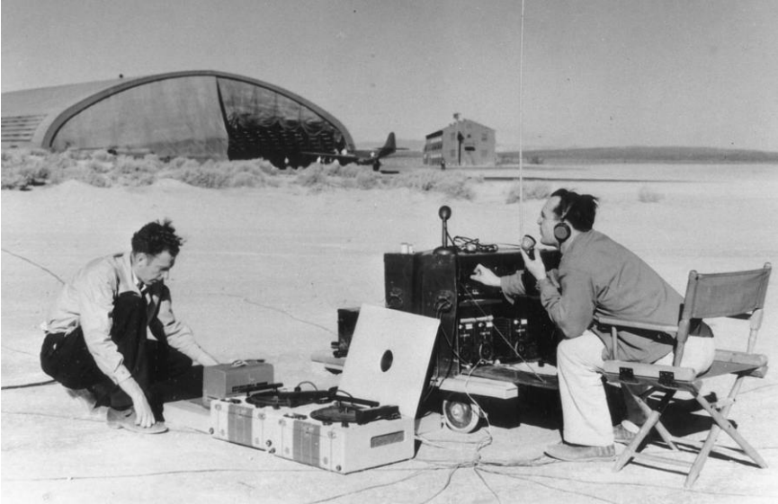
The original mission control center for the XP-59 flight test program consisted of a two-way radio and a wire recorder. The wires radiating out from the radio formed its antenna.
