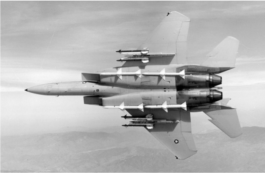
The large, low-mounted horizontal tail of the McDonnell Douglas F-15 Eagle is clearly visible in this view of the aircraft.
