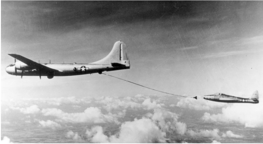
A KB-29 testing the British probe and drogue refueling system.
