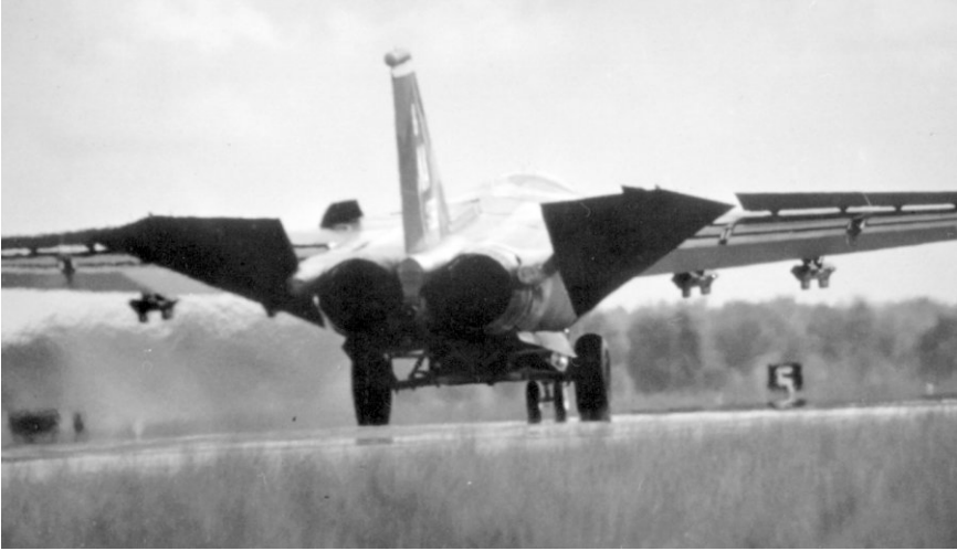
An F-111 landing, with wings swept forward and spoilers extended.
