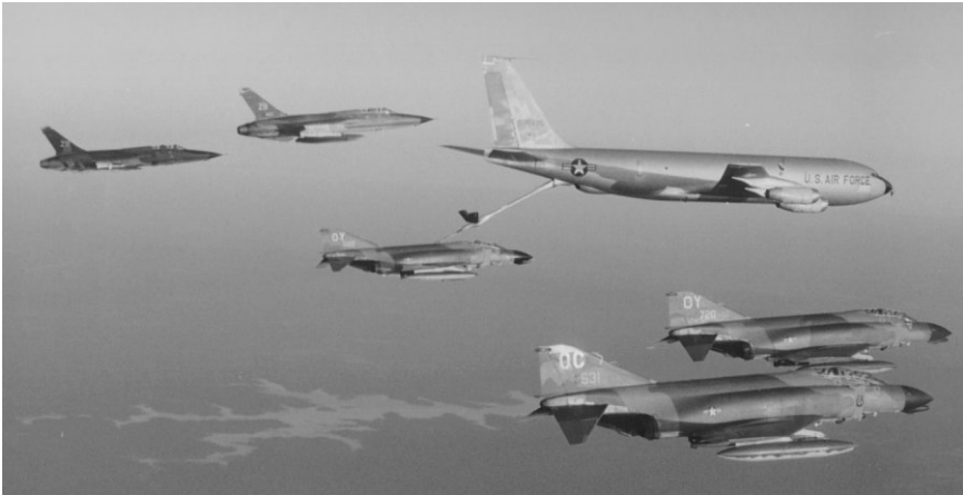
A KC-135 refuels an F-4 over Southeast Asia as four other fighters wait.
