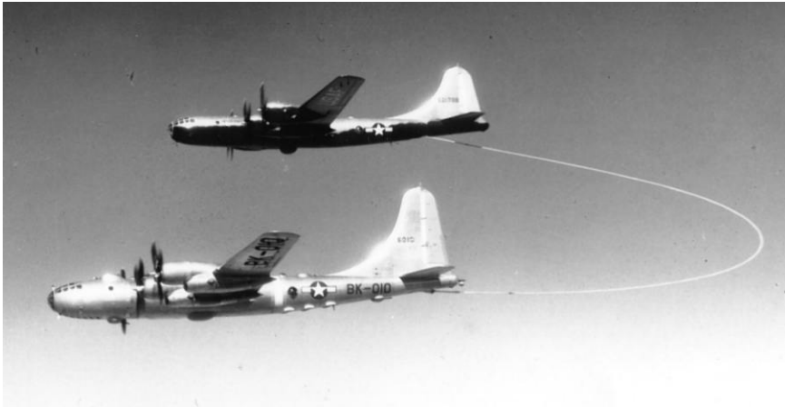
A B-50 receives fuel from a hose trailed from a KB-29.
