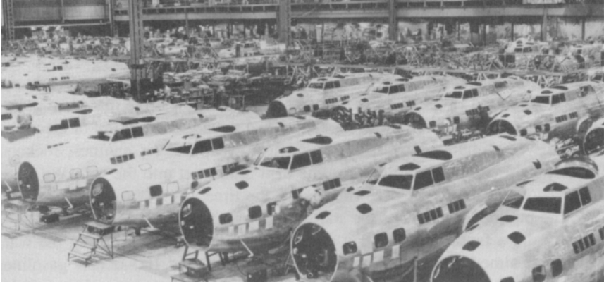
Approximately 7,000 Boeing B-17s were produced during World War II. This photograph shows fuselage sections under assembly.
