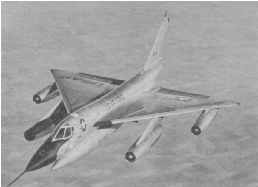
A delta-wing Convair B-58 Hustler with a ventral weapons pod. The Hustler was capable of speeds above Mach 2.
