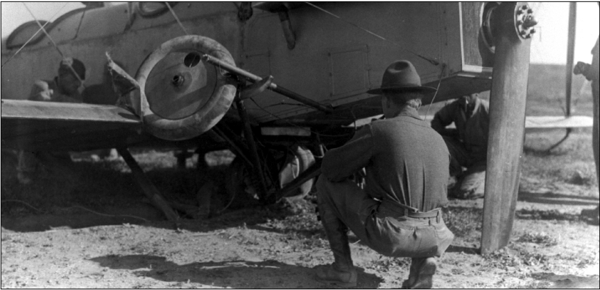
A rough landing wiped out the landing gear of this Curtiss R-2 at Columbus, New Mexico.
