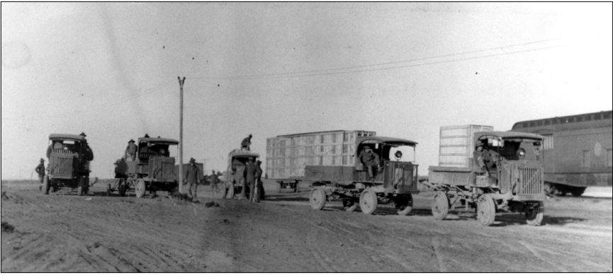
Transporting newly arrived Curtiss JN-4 aircraft from the rail head to the 1st Aero Squadron camp at Columbus, New Mexico, using Jeffery trucks, late 1916.
