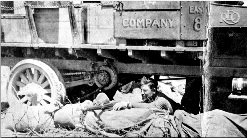
Prepared for an attack, a 1st Aero Squadron enlisted man takes his defensive position under a “REO” truck manufactured by the R.E. Oldsmobile Company. Note the chain drive, which was quite common to trucks well into the 1920s. (Vernon L. Burge Collection, Airmen Memorial Museum.)
