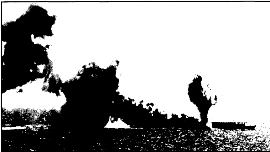
Japanese light carrier Shoho after attack by air units of the USS Lexington and the USS Yorktown in the Battle of the Coral Sea, May 1942. Built as a submarine depot ship, it was fitted with a flight deck, but to remain fast and maneuverable, it received no protective armor. Struck by bombs, torpedoes, and a crashing aircraft, it capsized and sank in just ten minutes.
