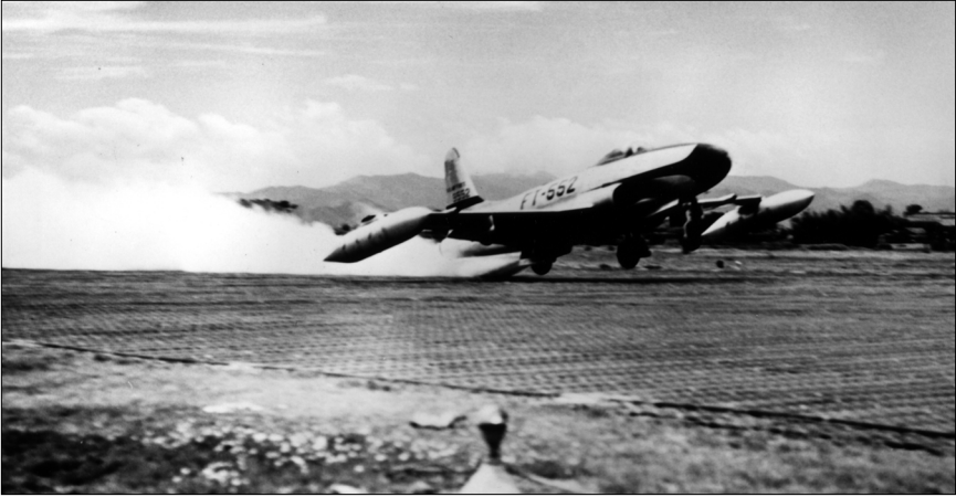
A heavily laden F-80 of the 51st Fighter-Interceptor Group makes a JATO takeoff.
