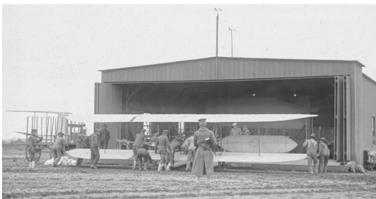
A Wright Model B, possibly the Collier Wright, is being assembled from a rail car at the top. Both panels of the right wing are in place. Inside the hangar at Fort Sam Houston are propellers, elevators, seats, wheels, rudders, and wings, awaiting assembly. The fully assembled Model B in the bottom photograph is being returned to its hangar.
