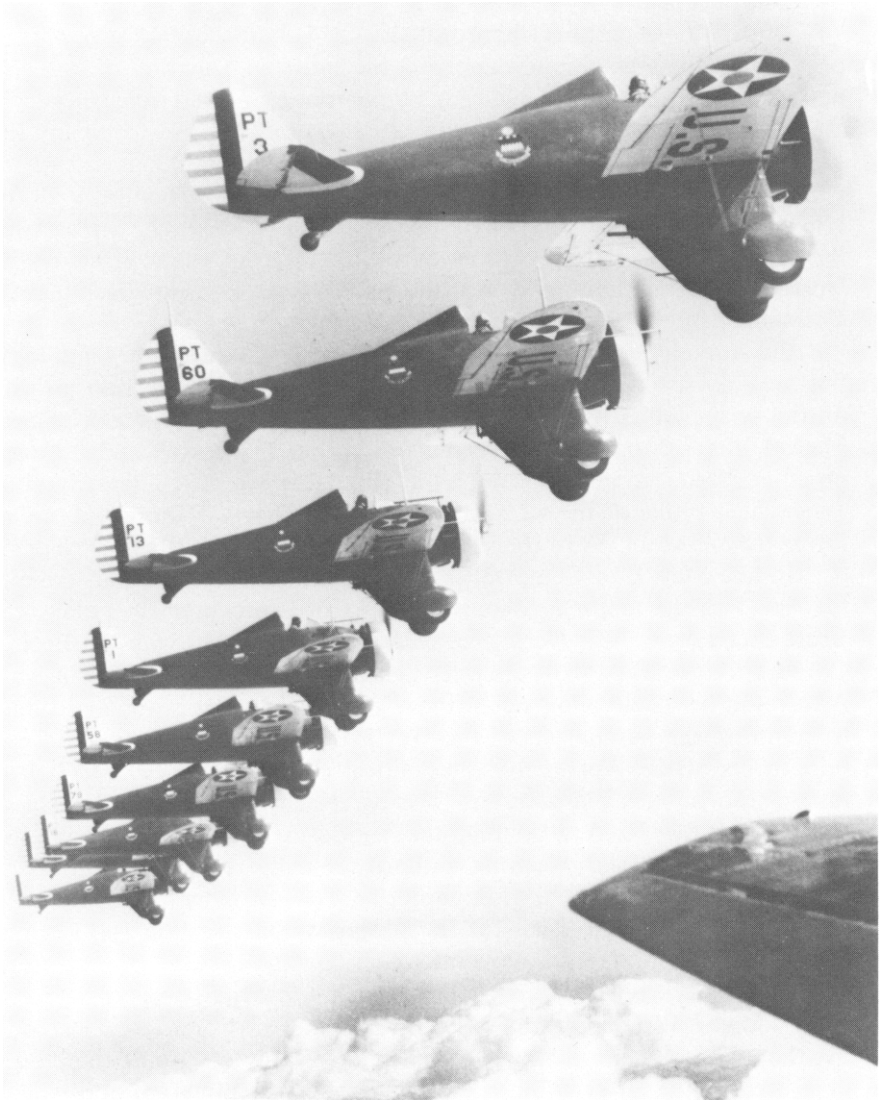
The P-26, which figured in some of Foulois' procurement trouble. This aircraft represented a major breakthrough in fighter aircraft design. It marked the historic change from wood and fabric to an all-metal monoplane fighter.
