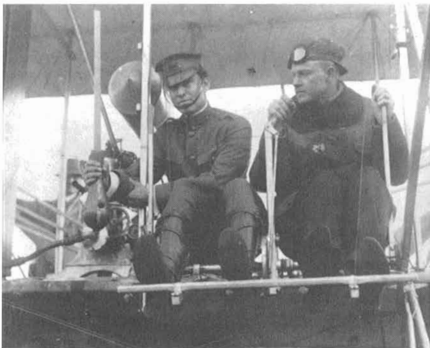
In the first such American experiment, Lt. Myron S. Crissy demonstrates a mechanical arm he devised to drop a 36-pound practice bomb from a Wright aircraft. Crissy hit a 20-foot circle on the Tanforan Racetrack, San Francisco, on January 15, 1911.
