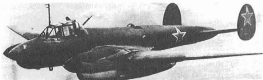
The Petlyakov Pe-2, a medium bomber, served as a dive-bomber early in the war.
