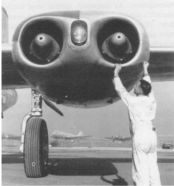
Close-up of 2 of the 4 jet engines that powered the XB-45.
