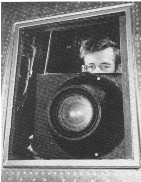
Looking in a port of a reconfigured RB-50B, one could see the lens cone of a hand-operated reconnaissance camera. This aircraft featured 9 such camera stations.
