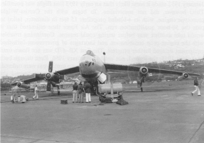
A specially modified Stratojet—the XB-47D—was used to test the Curtiss-Wright YT49 turboprop engine.
