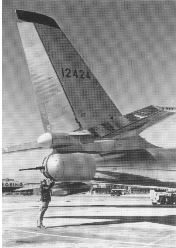
The radar-controlled tail turret of the B-47E featured twin 20-mm cannon.
