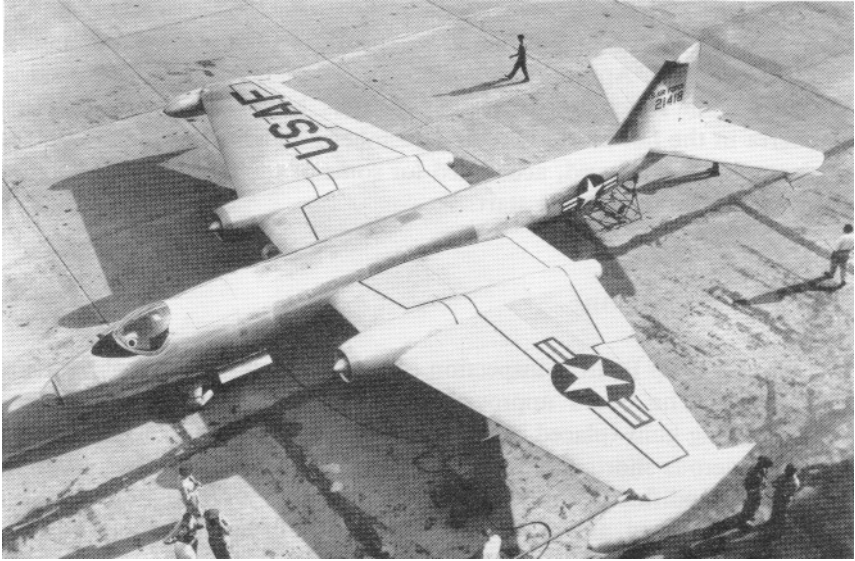
The B-57, an American version of the British Canberra, featured wing tip fuel tanks.
