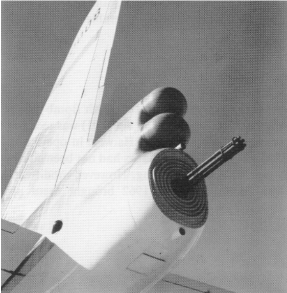
The ASQ-21 Gatling gun, mounted in the B-52H's tail, provided remote-controlled defense.
