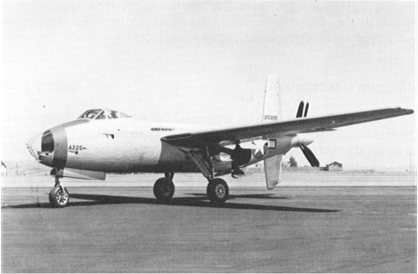
The XB-42 featured a novel engine-propeller arrangement.
