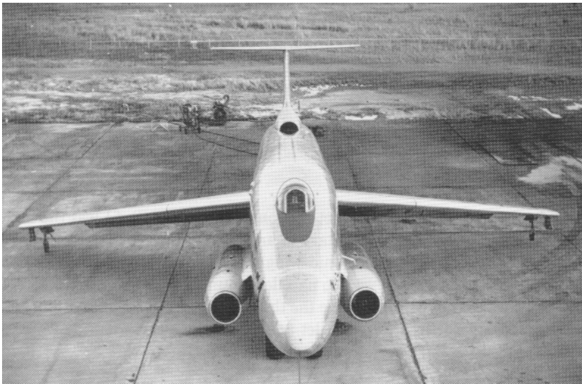
Two of the XB-51's turbojets were mounted on the fuselage. The third was inside the rear fuselage.
