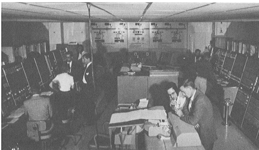
AN/FSQ-7 radar. Shown here is part of the maintenance control console of the central computer.
