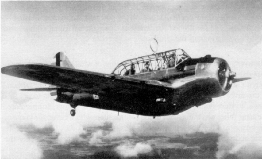
The three-place O-47 observation aircraft, which General Lee believes could not survive in the air against contemporary fighters.
