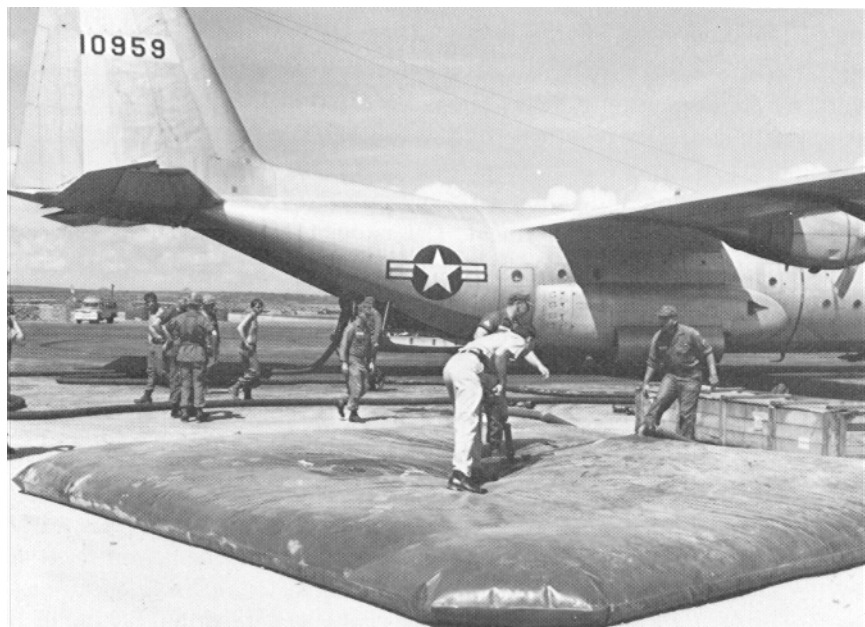
Aviation fuel is pumped from the fuel bladder aboard a C-130 into an empty bladder in a storage area at Phan Thiet, September 25, 1966.
