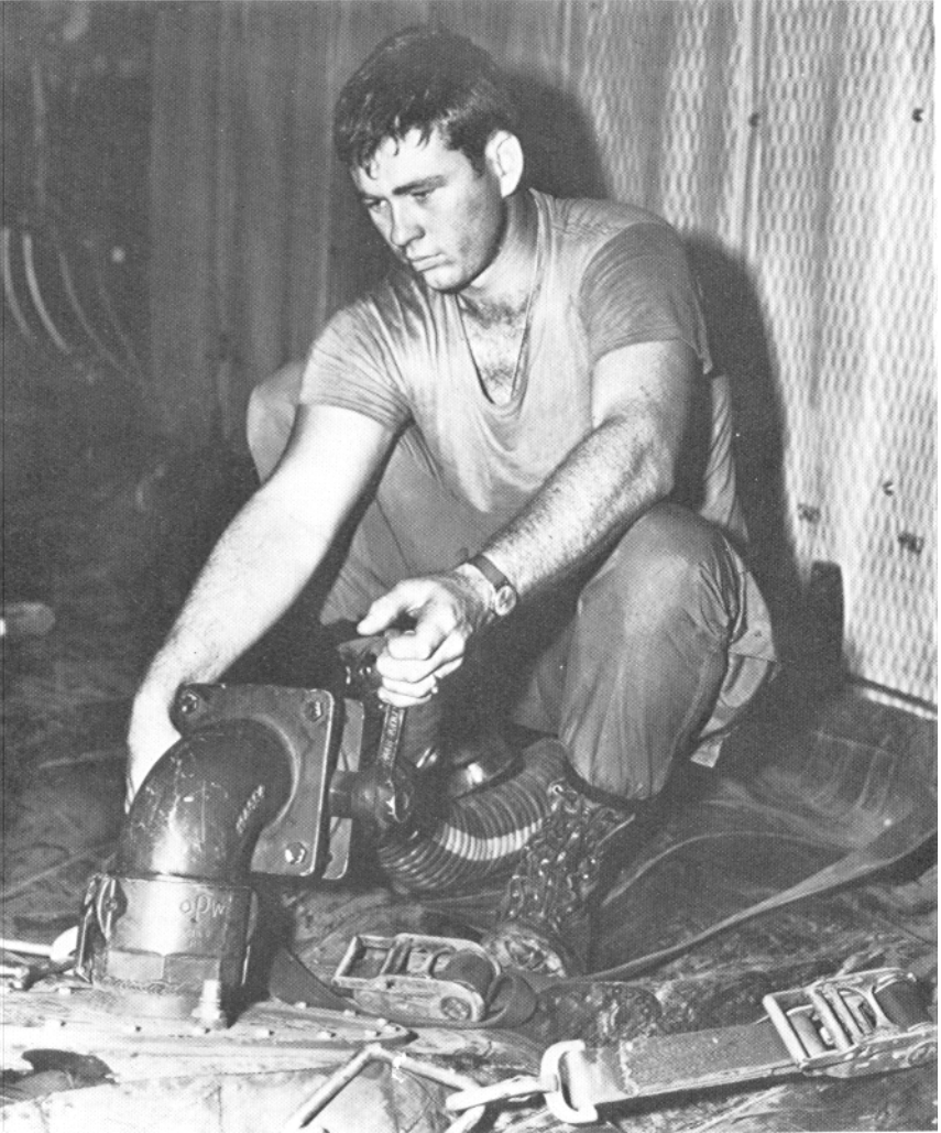
Sgt. Dannie B. Needham of the 377th Supply Squadron at Tan Son Nhut, checks a valve on a 6,000-gallon fuel bladder inside the C-130 aircraft.
