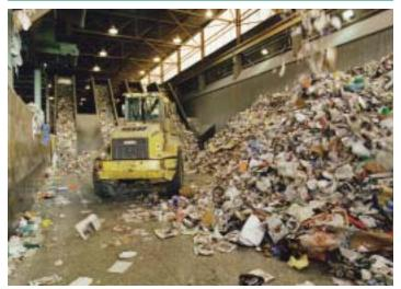
An end loader pushes the mixed recyclables onto four conveyors. The sorting plant uses sophisticated technology to separate paper from containers.
