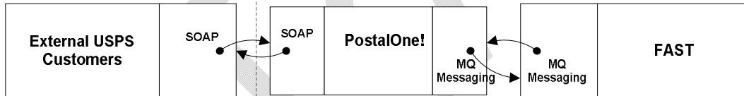
Figure 1-2. PostalOne! FAST Web Service Overview
