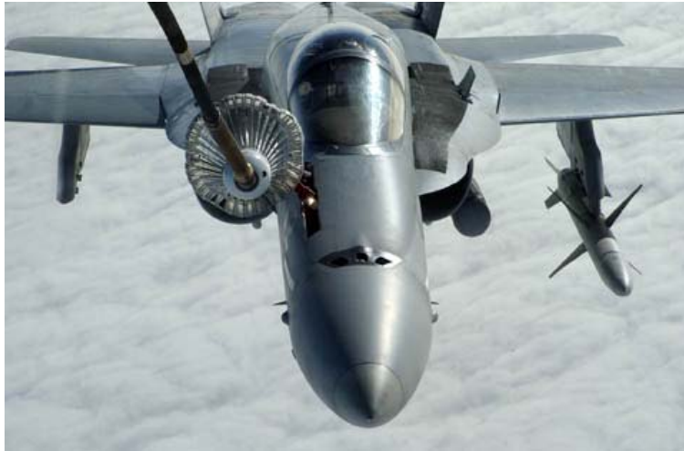
US Marine F-18 receiver aircraft using drogue air refueling procedures.
