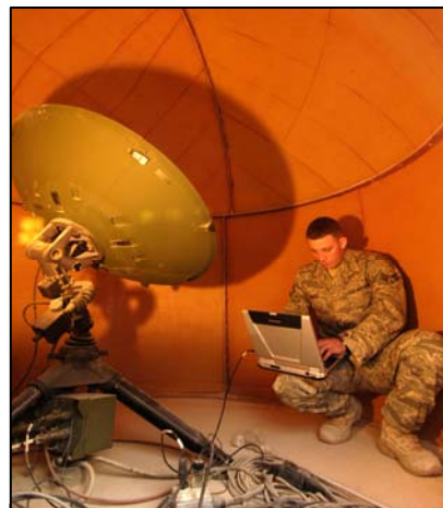
A U.S. Air Force network systems technician reacquires the Global Broadcast System, which is part of keeping an uninterrupted flow of information streaming to a Combined Air Operations Center.
