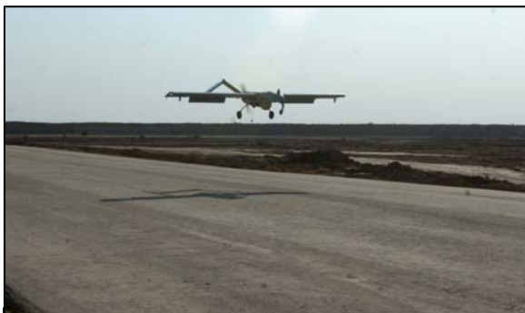
An RQ-7B Shadow (Group 3 UAS) begins its landing sequence following a flight to provide troops operating in Iraq with another set of eyes. Shadows are employed by the Marine Corps and Army.
