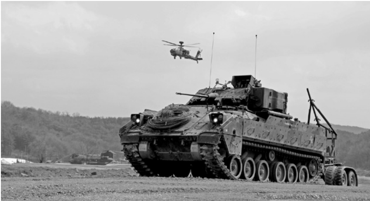
A Bradley Fighting Vehicle tows an M58 mine-clearing line charge as it prepares to clear a simulated minefield while an Apache helicopter provides fire support during the 2nd Infantry Division combined arms live fire exercise, 18 April 2010.
