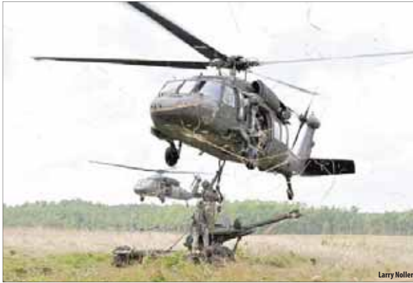
Soldiers from 1st Battalion, 320th Field Artillery Regiment, 2nd Brigade Combat Team, 101st Airborne Division connect lifting slings between M-119A2 lightweight towed howitzers and UH-60 Black Hawk helicopters from 5th Battalion, 101st Combat Aviation Brigade during training exercises at Fort Campbell, Ky., June 9. The process is complicated by flying debris kicked up by rotor wash.
