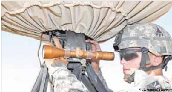
Pfc. Dustin Clark calibrates the sights on a radar system on Contingency Operating Base Basra, Iraq, June 28. Clark and other members of Battery E, 4th Battalion, 5th Air Defense Artillery Regiment, out of Fort Hood, Texas, detect mortar and rocket attacks.
